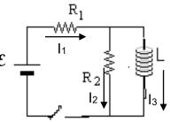
**23.** For the circuit used in the previous problem, find the current through resistor  $R_1$  at time  $t = \infty$ , after the current through the inductance has reached a constant value.
