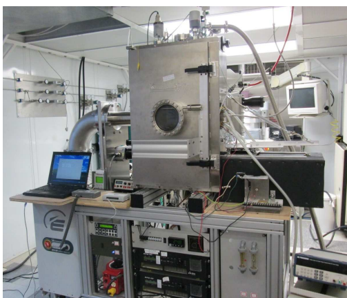
Figure 1. Photo of the hollow cathode sputtering system at NJIT.
