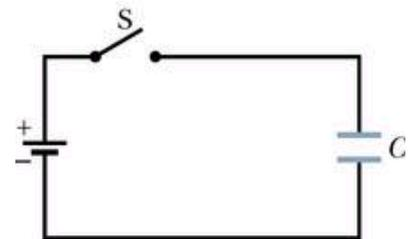
10. A parallel plate capacitor being designed is supposed to have a capacitance of  $400 \text{ pF}$  ( $1 \text{ pF} = 10^{-12} \text{ F} = 10^{-6} \mu\text{F}$ ). It will be filled with a material whose dielectric constant is close to 1.5 (glass). The distance between plates will be  $0.3 \text{ mm}$ . Approximately, what should the area of the plates be?
