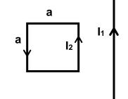
**14.** For the previous problem, calculate the magnitude of the force which acts on the frame if the distance from the straight wire to the closest side of the square is also 0.2 cm = a.
