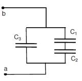
In problem 6, calculate the voltage across capacitor C2 (in volts)
